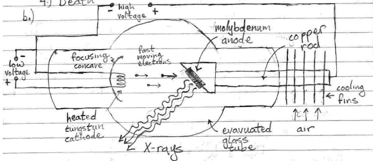
The heated tungsten cathode causes thermionic emission of electrons. These fast moving electrons strike the molybdenum anode. Electrons in the molybdenum absorb the energy of the fast moving electrons, and they move up to higher energy levels. As these electrons fall back to lower energy levels they emit X-rays.
