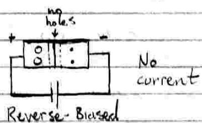
When the diode is forward-biased the holes in the P-region move toward the N-region, and the electrons from the N-region move across: current flows. When the diode is reverse-biased the
