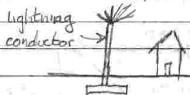
The lightning conductor is used to safely allow lightning to flow to the ground by providing a path of low resistance.
