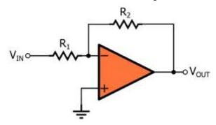
A well-labeled diagram of an operational amplifier in inverting mode should be drawn, showing the input resistor, feedback resistor, and output voltage.
