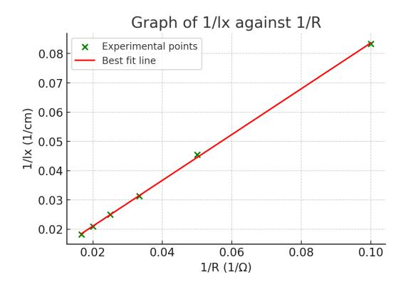
From the tabulated data, a graph of  $1/l_x$  on the y-axis against 1/R on the x-axis is drawn. The plot is expected to be a straight line.
