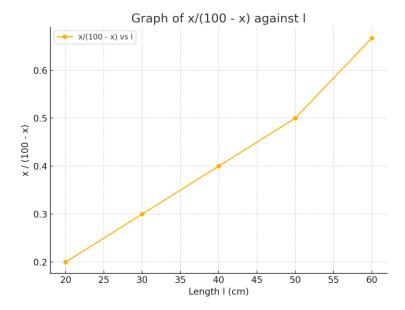
(f) Using your graph, determine the resistance per centimeter of the wire L, and the value of resistance P.
