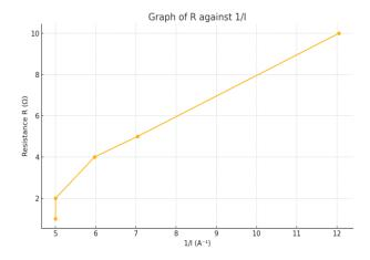
Use two points: (5.000, 1) and (12.048, 10) Slope =  $\Delta R / \Delta (1/I) = (10 - 1) / (12.048 - 5.000) = 9 / 7.048 = 1.276$ Intercept =  $R - S \times 1/I = 1 - (1.276 \times 5.000) = 1 - 6.38 = -5.38$
