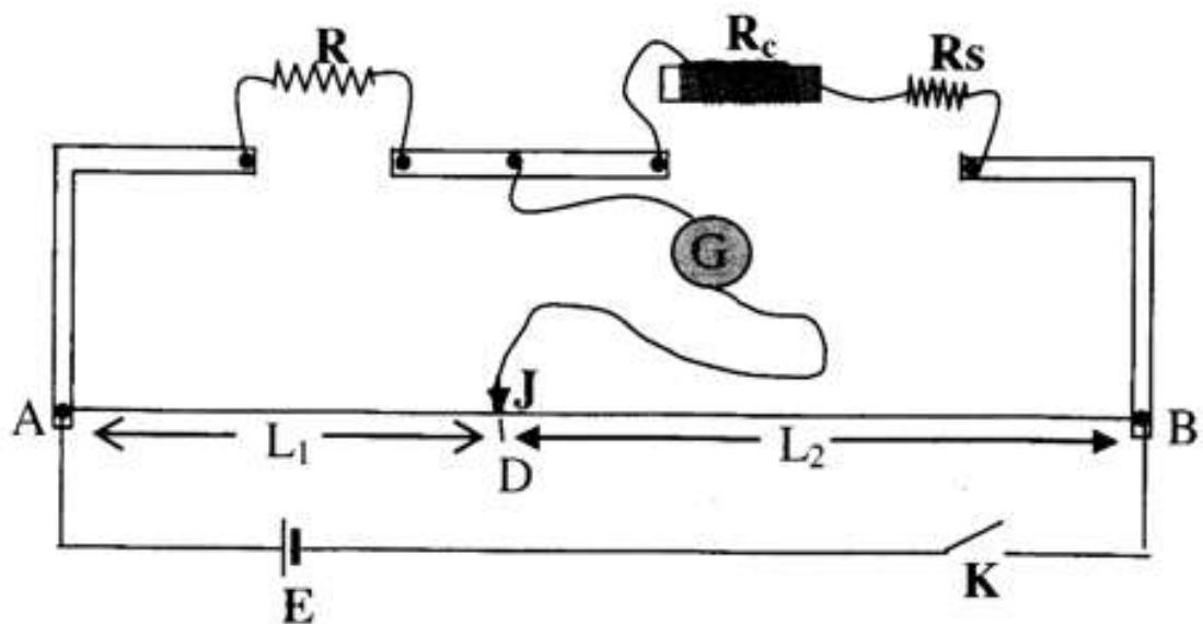
(b) Set  $R=1\Omega$ , close the key, **K** and determine the balancing point **D**. Record the lengths,  $L_1$  and  $L_2$
