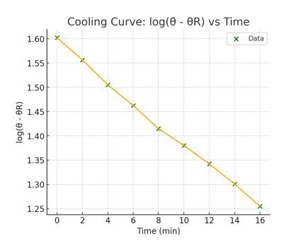
(iii) Slope represents the cooling constant, related to heat loss rate in pipes from heater to bathroom outlets.
