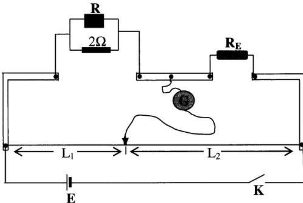
(a) Starting with  $R = 10 \Omega$ , close the key, K and determine the length,  $L_1$  where by, the galvanometer reads 0 and hence determine the corresponding value of length,  $L_2$ .
