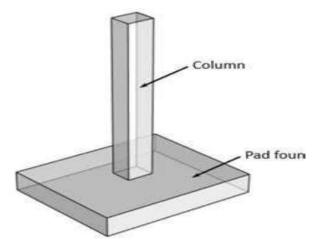
A pad foundation is a type of shallow foundation that supports and distributes the load of a single point load, such as a structural column, to the ground. It consists of a concrete block, typically square, rectangular, or circular in shape, placed beneath the load-bearing element. The primary purpose of a pad foundation is to spread the load over a sufficient area of soil to prevent excessive settlement or bearing capacity failure.
