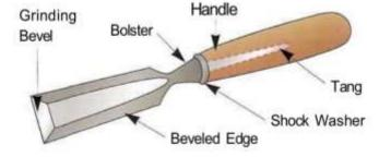
A skew edge chisel consists of the following parts:
