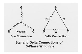
In a star connection, one end of each of the three windings is connected to form a neutral point, and the other ends are connected to the respective phase lines.
