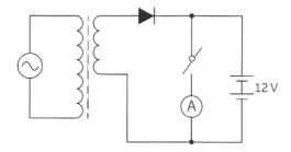
(The diagram includes transformer, single diode, battery, switch, ammeter in series, and AC input. Image can be generated.)
