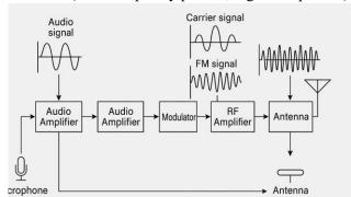
6. Antenna – Radiates the FM signal as electromagnetic waves.
