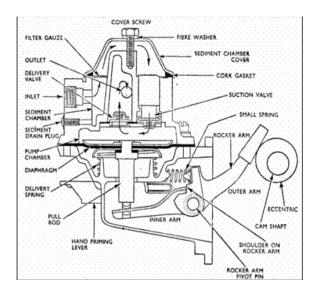
(b) Mechanism of the mechanical fuel pump.
