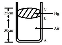
The above diagram shows a vertical uniform tube containing a mercury thread CB and a volume of air AB.
