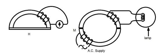
Figure H above shows a \(\cap-\)-core of iron with a coil wound on it. The ends of the coil are joined to a galvanometer. What would you notice in the galvanometer if you put a bar magnet on the core and took it off? (2 marks)
