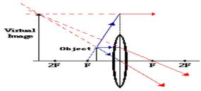
Ray Diagram for Object Located in Front of F
