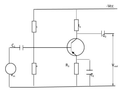
Resistors  $R_1$  and  $R_4$  are potential dividers
