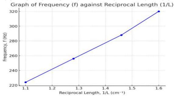
the graph of frequency (f) against reciprocal length (1/L). The linear trend confirms the direct proportionality between frequency and reciprocal length.
