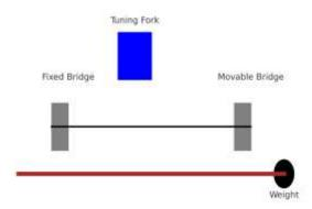
This is the sketch diagram for the sonometer experiment setup. It includes a fixed bridge, a movable bridge, a tuning fork placed above the vibrating wire, and a weight at the end to maintain tension.
