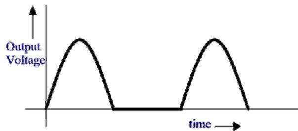
(ii) The semiconductor diode, when connected as above is not suitable for use in a radio because the output is intermittent and hence will introduce interference in the radio signal.
