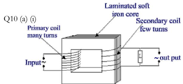
A step down transformer consists of a laminated rectangular soft iron ring on opposite arms of which are wound the primary coil with many turns through which the input voltage is fed. On the opposite arm of the laminated soft iron core is wound a secondary coil with fewer turns from which the output with lower voltage is drawn. The wire in the secondary coil should be thicker than that in the primary coil so as to be able to carry the higher current which will flow in the output circuit.
