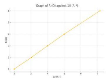
Plot R on the y-axis and 1/I on the x-axis. The graph is expected to be a straight line because from the equation E = I(R + Q), we get:
