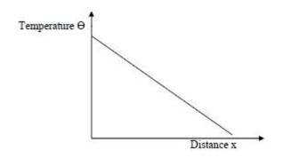
(b) Deduce the rate of heat flow through a plaster ceiling, measuring 5 m  $\times$  3 m  $\times$  15 mm, in contact with 45 mm thick layer of insulating material. If the inside and outside surfaces are at the surrounding air temperature of 15 °C and 5 °C respectively, the thermal conductivity of plaster ceiling is 0.60 Wm<sup>-1</sup>K<sup>-1</sup> and that of insulating material is 0.040 Wm<sup>-1</sup>K<sup>-1</sup>.
