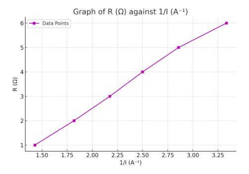
(iii) Using the graph and the equation  $R = (E \times 1/I) - r$ . Find the value of E.
