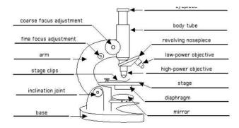
(ii)part E is the mirror whose function is to reflect light on the stage in order to enable good observation of the specimen.
