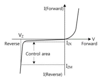
The characteristic curve of a zener diode shows the forward region (normal diode behavior) and the reverse breakdown region, where the diode conducts in reverse to regulate voltage.
