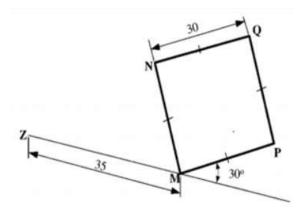
2. The figure below shows a hard plastic engine mounting require by a Car Company. By using full size scale and isometric projection; construct a free hand sketch of a part.
