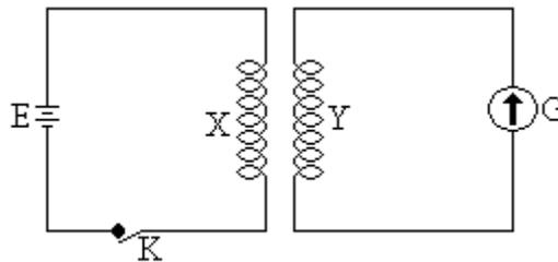
(i) State and explain the deflection of the galvanometer needle when the switch K is closed for a few seconds and then opened.
