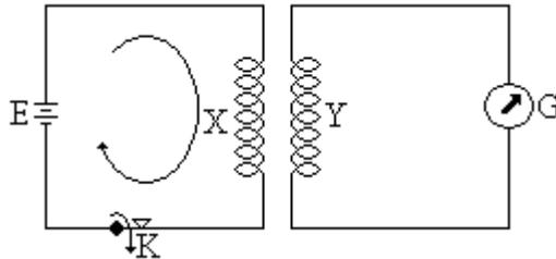
If switch K is closed the galvanometer will deflect and then return to zero. When switch K is opened the galvanometer will deflect in the opposite direction and then return to zero. Deflection happens when K is opened and closed because this is when the flux changes in X and Y since the induced e.m.f depends on the rate of change of flux
