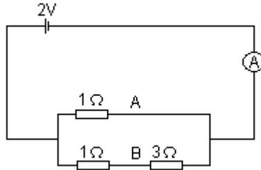
Since part A and B are in parallel, you will add their inverse. In part B there are two resistors in series, so their resistances will be added
