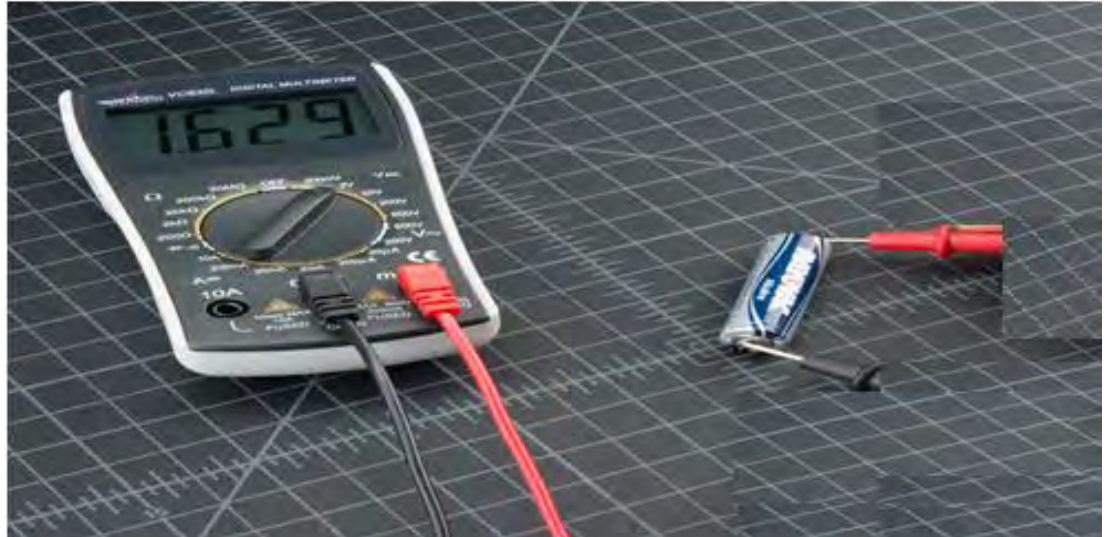
Figure 6: The value of voltage V on an AA battery
