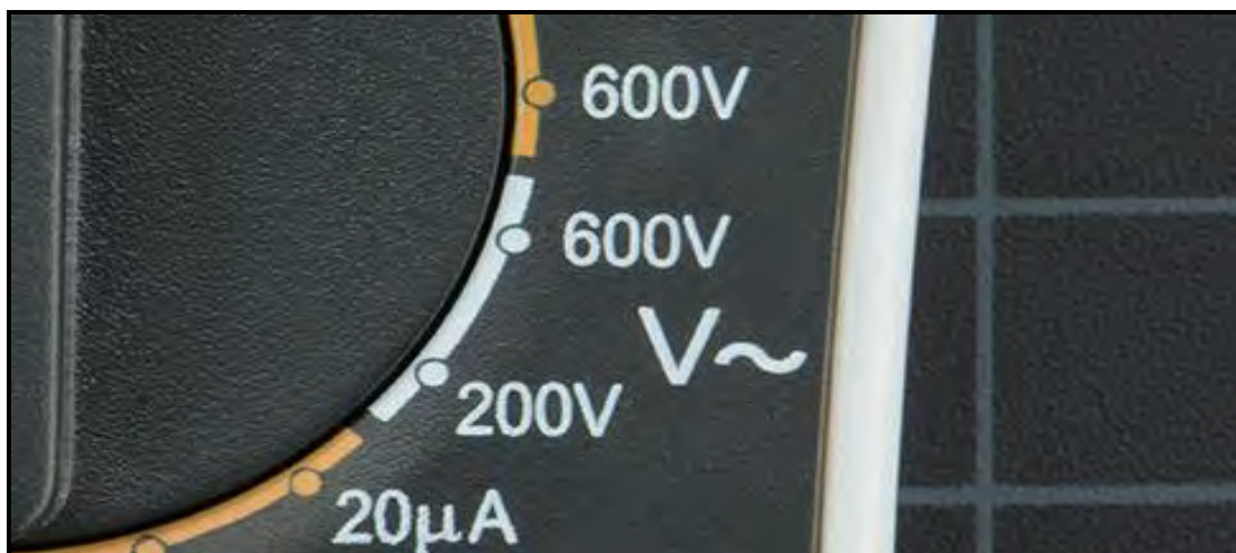
Figure 8: Use V with a wavy line to measure AC Voltage
